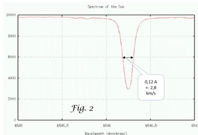
In Figure 2 we can see the double scattering of the brightness of the spectral line according to Gauss  $2\sigma = 0.12 \text{ A}$  (Angstrom). The scatter ( $\sigma$ ) of the brightness of the spectral line is therefore  $0.06 \text{ A}$ .
